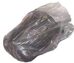
BMC – Pre-peg Charge in High Barrier Bag
